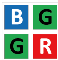
Figure 11-11 Bayer BG Pixel Pattern
