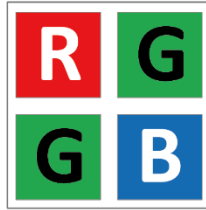
Figure 11-12 Bayer RG Pixel Pattern
