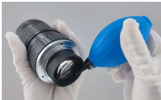
Figure 2-1 Cleaning by Rubber Dust Air Blower
