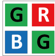
Figure 11-9 Bayer GR Pixel Pattern
