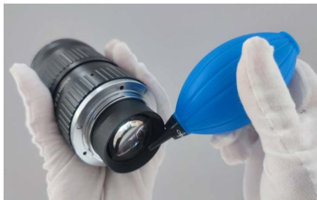
Figure 2-1 Cleaning by Rubber Dust Air Blower
