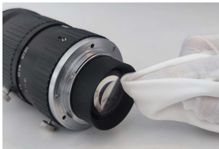
Figure 2-3 Cleaning by Lens Cleaning Paper
